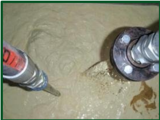
Holding tote pump and return lines with solution.
