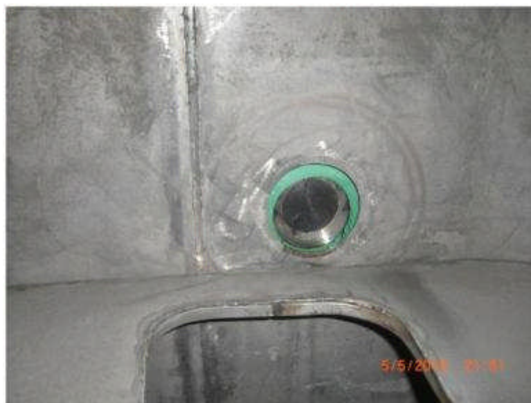
Internal of 60 gallon reservoir after chemical flush
