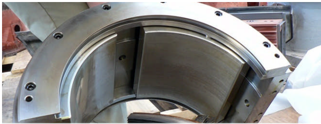
Clean Bearing Pads found After ESP Installation
