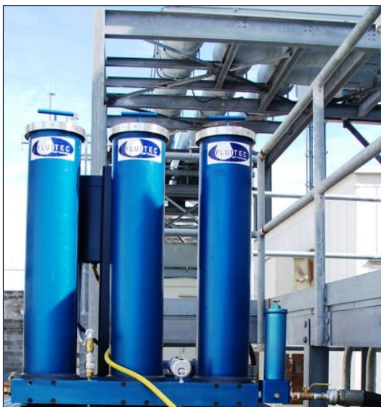
ESP-336 being rotated around a combined cycle plant to maintain 4 turbine oil reservoirs
